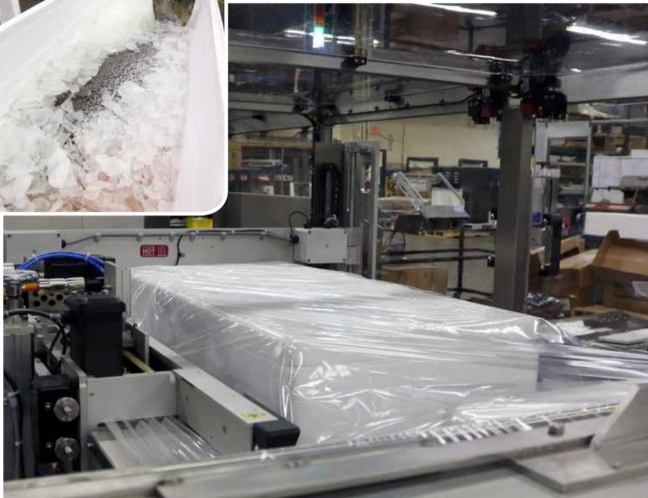
The fully-automatic Damark B34/180 HS-SS-N4 shrinkwrapping system manufactured by Plexpack is designed to wrap 27 Styrofoam containers, filled with varying loads of fresh salmon and blocks of dry ice to keep the fish fresh during transit, per minute.
