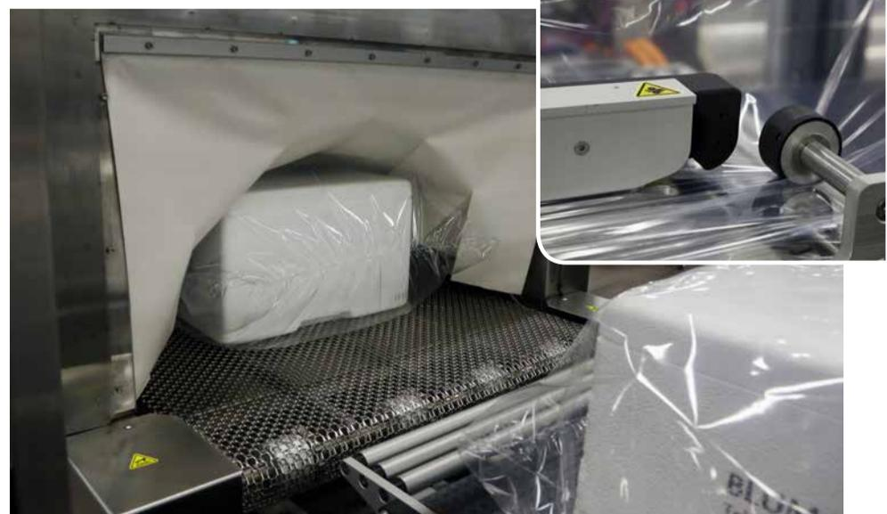
After being fully wrapped around all sides with the protective film, the Styrofoam containers make their way into the system's high-performance heat tunnel to have the film shrunk tightly around all of the container's contours without any tears or air bubbles.
