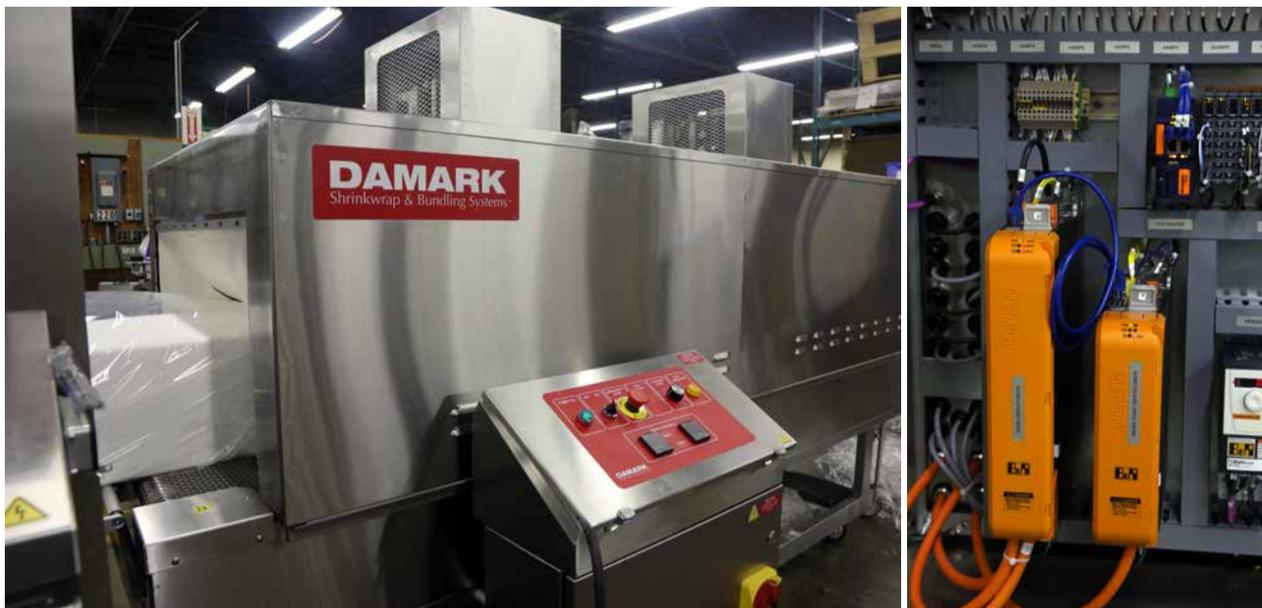
The Damark shrinkwrapping system manufactured for a leading South American salmon producer incorporates leading-edge automation components and controls, such as the high-efficiency servo drives from B&R Industrial Automation (inset), to provide the client with a highly robust and reliable end-of-line packaging solution.
