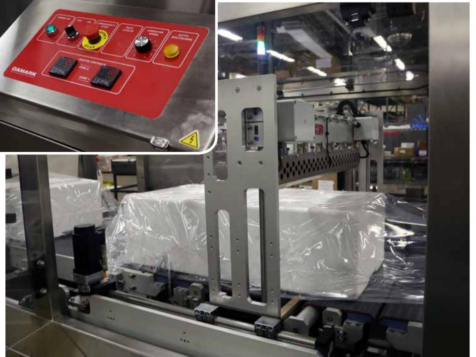
Featuring user-friendly machine controls and status indicators (inset) to facilitate simple plug-and-play operation, the custom-made Damark machine wraps the Styrofoam containers with high-strength clear polyolefin film before transferring them into the heat tunnel.
