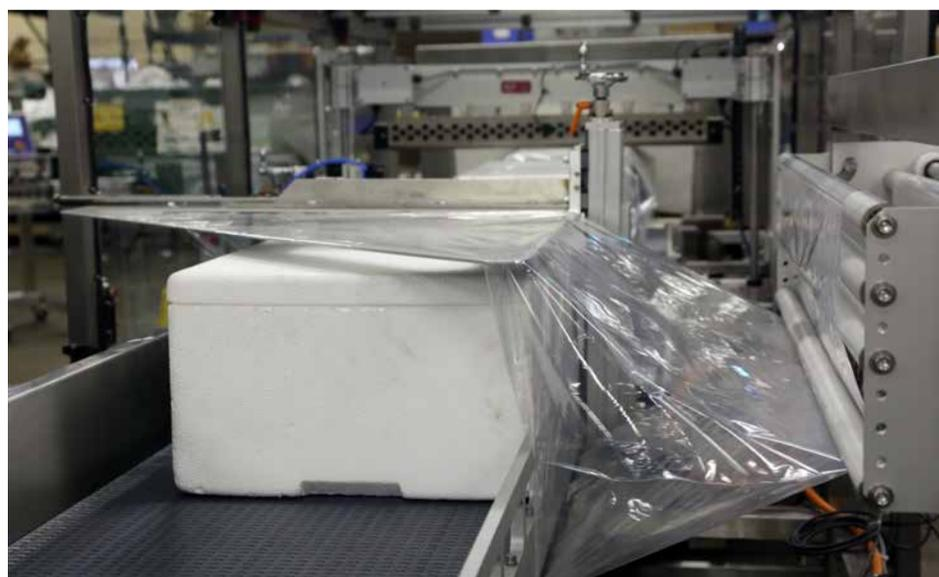
The custom-made Damark shrinkwrapping line uses the company's proprietary continuous-sealing technology to wrap the protective polyolefin film layer around each foam container in a highly secure cross-seal pattern to ensure complete coverage around all sides.
