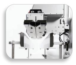
an all-in-one automated solution for a wide range of dry flowable, weigh/count applications. The ABS combines robust, stainless steel bag sealers with food grade bag presenters, hoppers, spouts and conveyors to produce hermetically sealed packages weighing up to 10 lbs (4.54 kg) and up to 12" (30.48 cm) wide and 16" (40.64 cm) tall.
