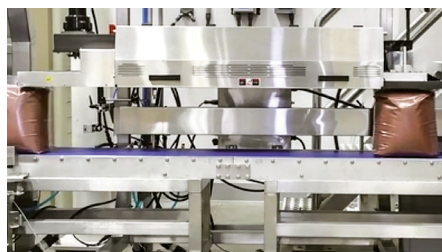
MPS 14000 NEMA 4-rated model bagging salt.
